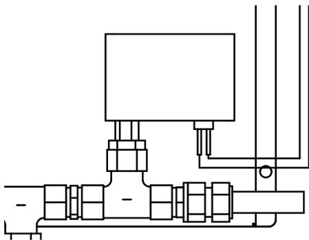
Range left hand scale should be set at 5 bar (75 psi) and differential at 1.5 bar (23 psi). Use adjuster screws on top of pressure gauge to adjust if required.
