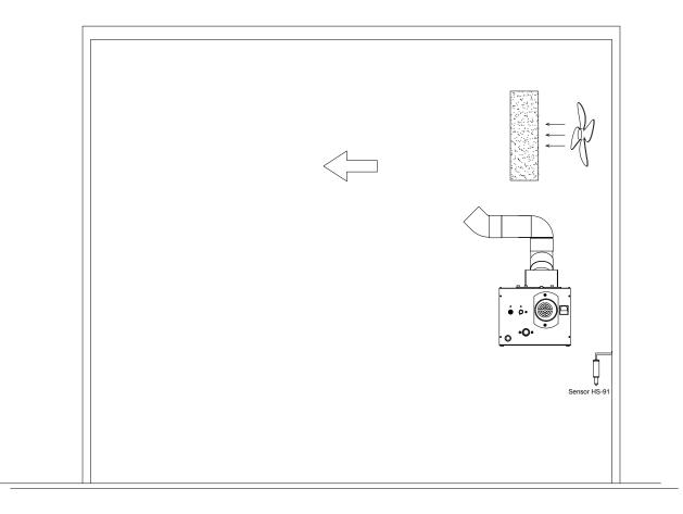
• The humidifier and R.O. equipment should be installed inside a coldroom in the following conditions: RH < 99%
