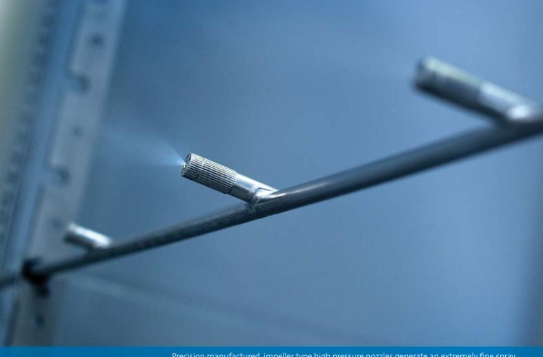
Precision manufactured, impeller type high pressure nozzles generate an extremely fine spray
