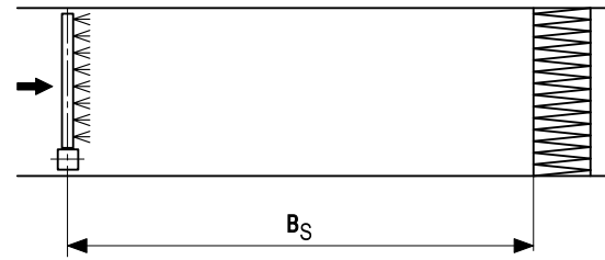
Fig. 33: Installation in duct Downstream obstacle: Particulate filter
